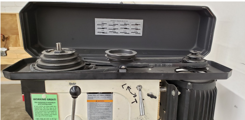
Belt Tension Lever - Adds or removes tension from the drive belts
