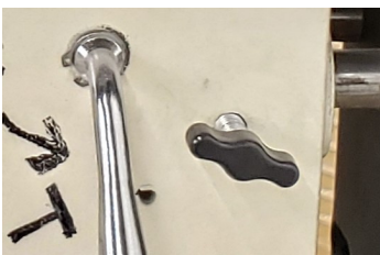
Belt Tension Locks - Locks the belt tension in place
