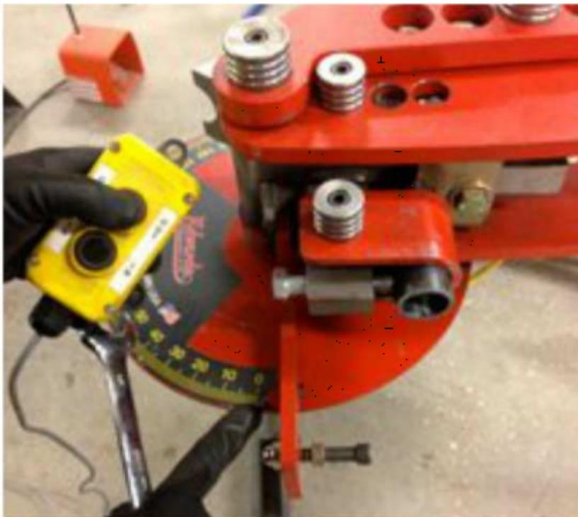
Now press the remote OUT button to start the bend. When you reach the end of the first step, jog the bender back with the IN button to make it easier to remove the step pin. Now adjust the step pin to the next hole in the die to finish the 90-degree bend.
