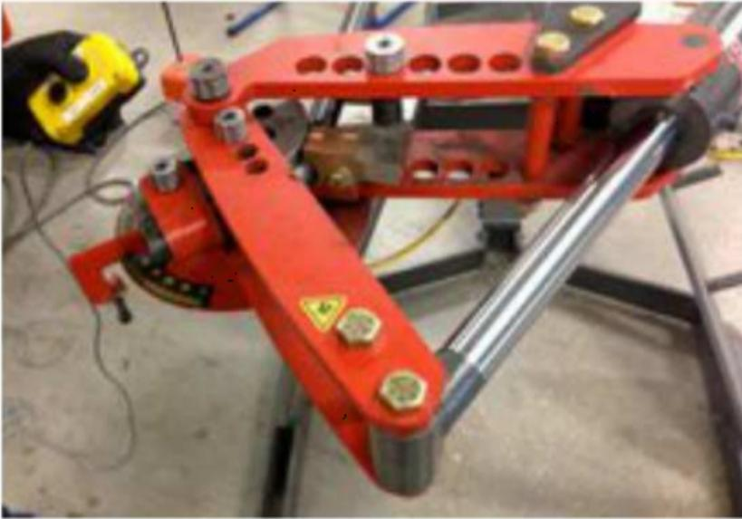
To safely remove your pipe, jog the bender back using the IN button to relieve the pressure on the pipe. Remove the collar, step pin and backstop to remove your pipe.
