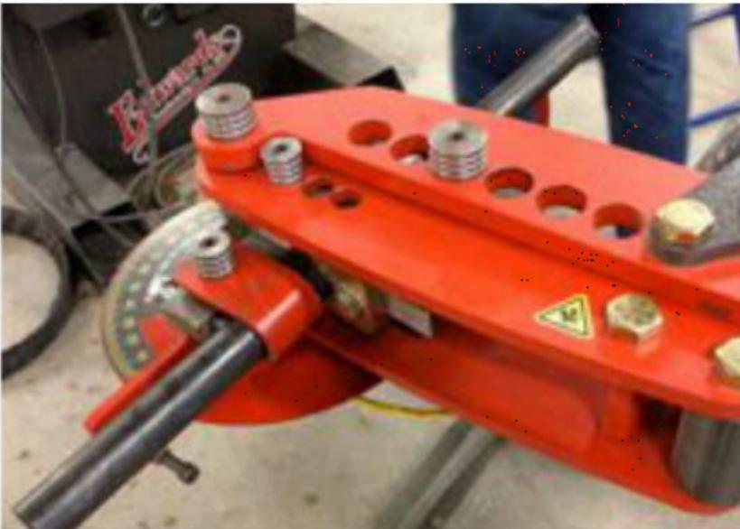
**NOTE:** If you are making a bend at the end of a piece of pipe you want to make sure that it is even with the end of the die.
