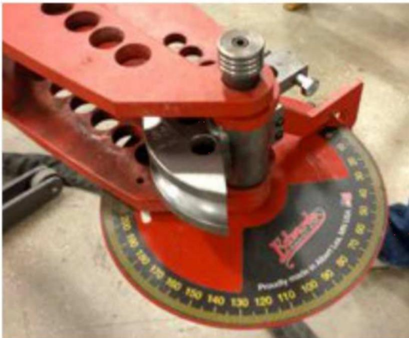
Next, take your backstop that matches the die and install it on the non-moving arm of the bender with another pin. Make sure that the screw is towards the bottom of the bender.
