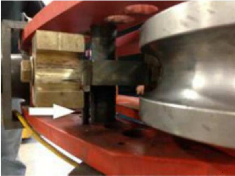
Now you can slide your pipe into the bender between the die and backstop. The collar that holds the pipe goes on next using the short pin.
