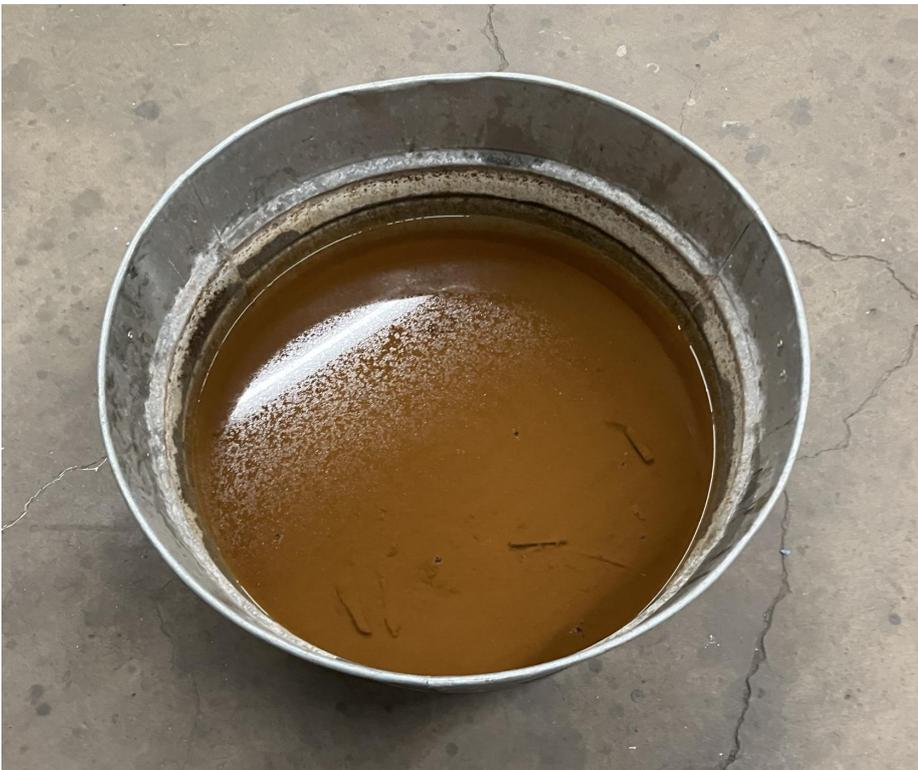
The quench tub is used to quickly cool tools and forged workpieces.
