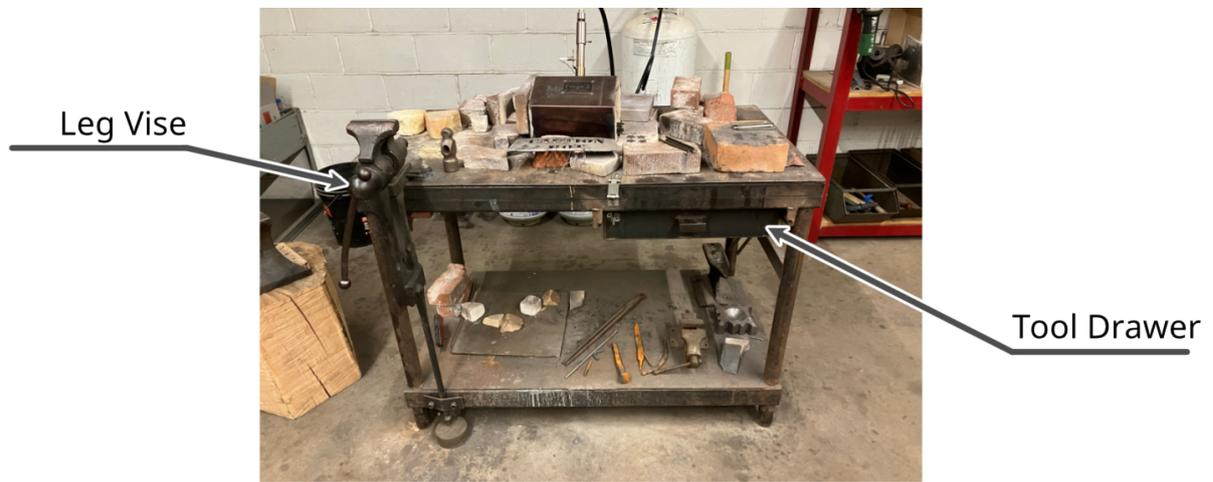
The large forge table can be used to rest heated workpieces and tools.
