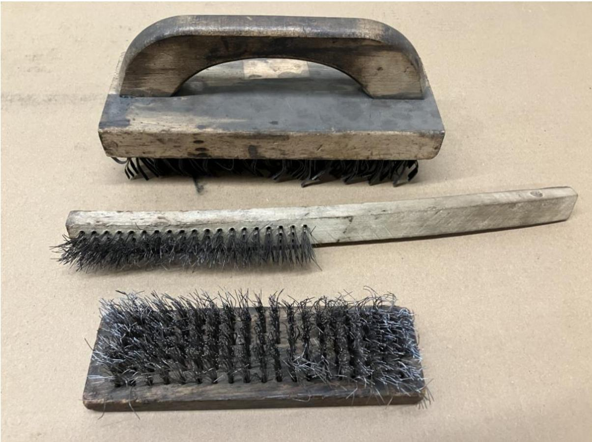
Brushes are used to clean the scale off of forged material.
