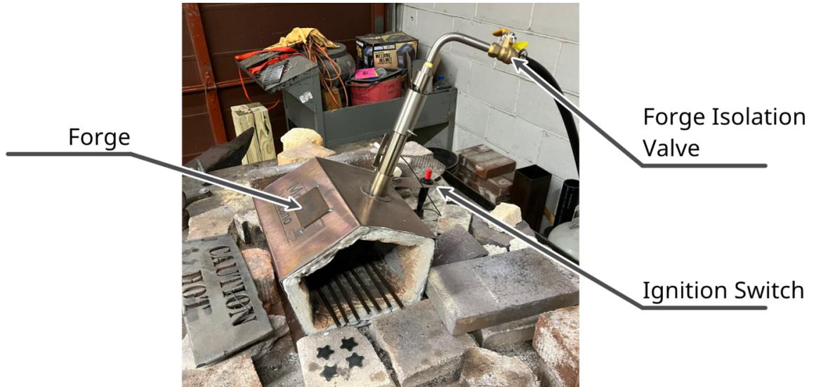
The firebrick inside the forge protects the refractory material from damage.
