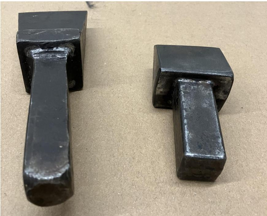
Only use a hardie tool if it fits *loosely* in the hardie hole of an anvil. You may need to use a different anvil for a particular tool.
