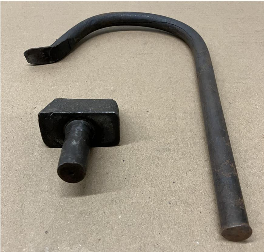
Holdfasts are hung from the large forge table. Holdfasts can be used in pritchel holes to hold a workpiece to the anvil.
