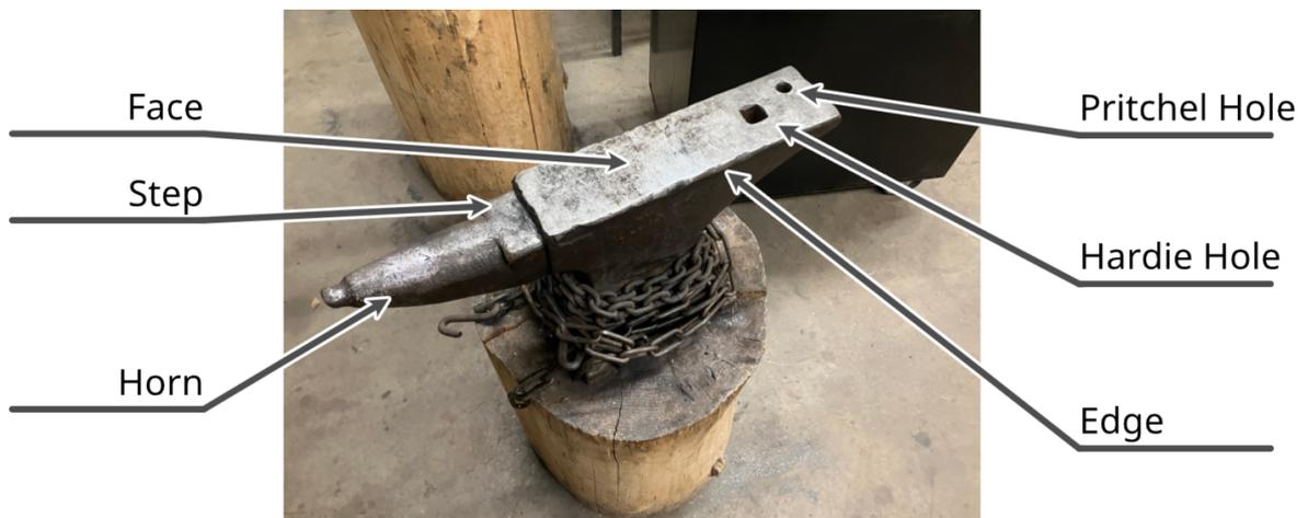
**Face.** The face is the flat area at the top of the anvil. The top of the face is used to flatten and shape material. The edge of the face can be used to bend material. Face edges can be sharp or rounded to achieve different kinds of bends.
