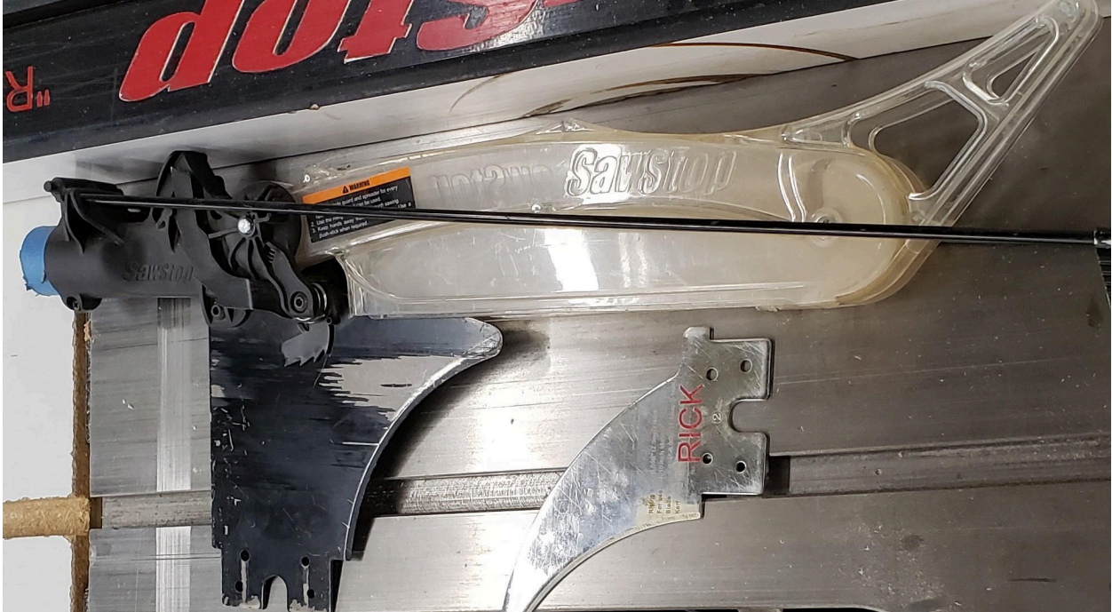
7. Riving Knife - Used as a splitter that follows the height of the blade. Must be installed if not using the blade guard.
