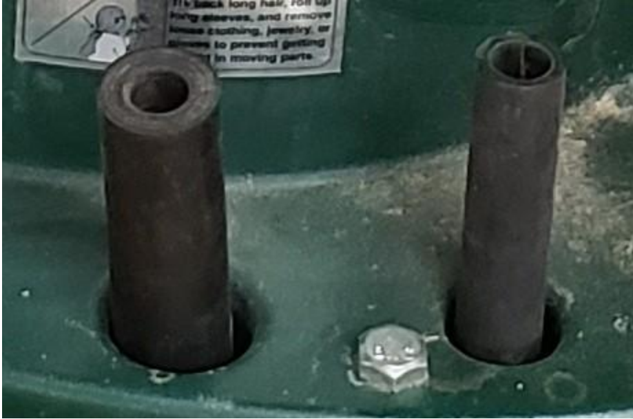
4. Abrasive Sleeves - These consumables slip over the drums.
