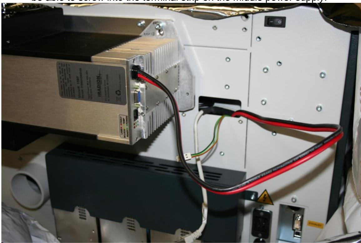
Terminal strip on the middle power supply with laser wires (thick red and black wire should be removed).
