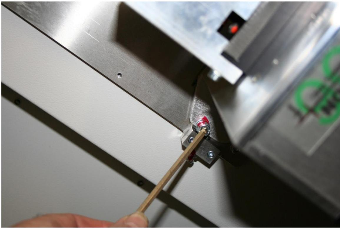
Remove connectors from laser. The black and red wires that travel from the laser into the opening in the back of the engraver and out through the bottom so as to be able to screw into the terminal strip on the middle power supply.
