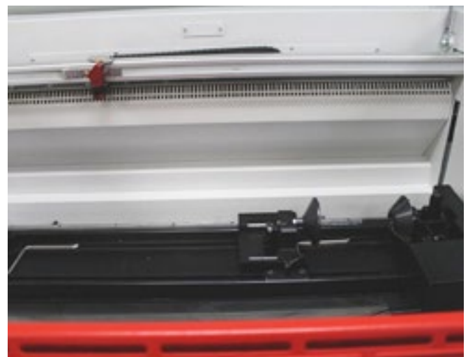
Place the pointed cone on the right for tapered items
