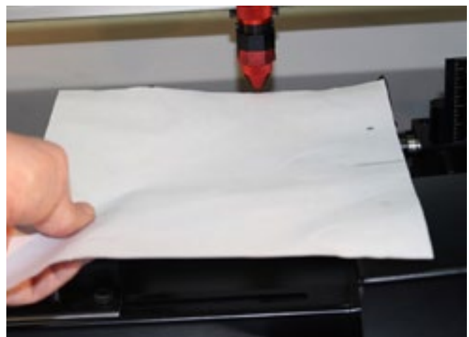
Top of the page stops at top center of rotary fixture
