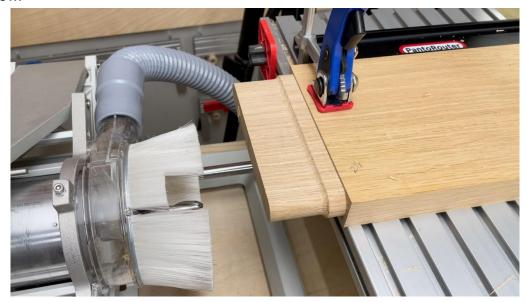
2. Leaving the work piece in place, we then used a 3/4" bearing-guided roundover bit to go around the front edge to soften it
