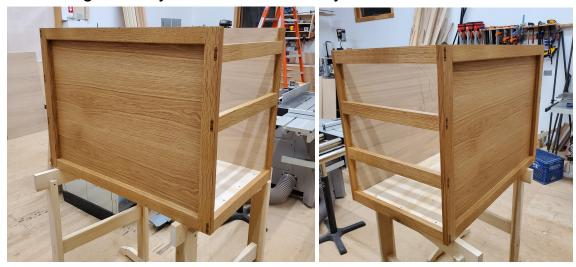
10. Mill and glue the wood for the top of the cart. We used scrap that we had around the shop leftover from previous projects. We decided to cut 3 mortises in the top's overhang to hold the PantoRouter clamps as well as router collet wrench(es) in order to keep these close by.
