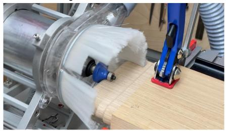
3. The piece was then placed on the tilted table to cut the finger pull on the underside using a box core bit. This slight angle makes a really comfortable hand hold. This cut goes across the entire bottom on the tenon. The Slot Mortising template was used for this operation
