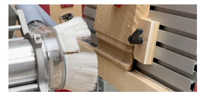
4. Next the profiled piece was cut off of our longer piece of wood. It was sanded and the edges were softened by hand.
