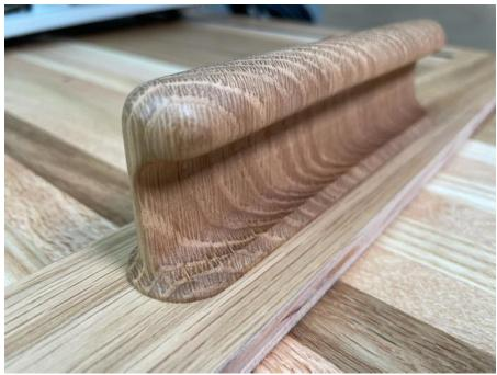
5. Lastly, a corresponding mortise was cut in the drawer faces to accept the tenon of the drawer pull. The drawer pull was then installed into the drawer face and the whole thing got a couple coats of finish. The result is a really clean look that adds a nice level of detail to the cart and it's easy to do using the PantoRouter™.
