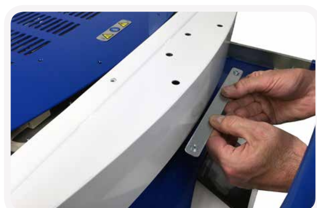
Replace bracket with bushes on the top side.
