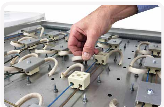
Fitting the new element is a reversal of the previous procedure.
