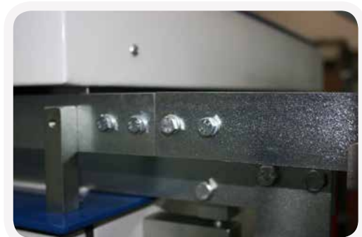
Refit and tighten the screws through the rear heater rail and into the links.
