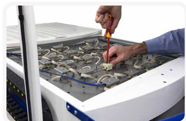
Tighten all connections securely.
