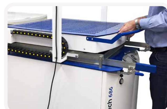
Replace heater cover and tighten all 16 screws.
