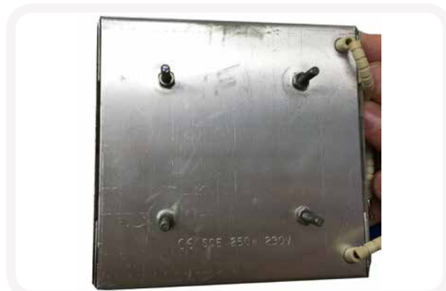
Element case showing wires and four securing bolts. It also shows the wattage + volts.
