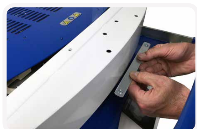
Replace bracket with bushes on the top side.
