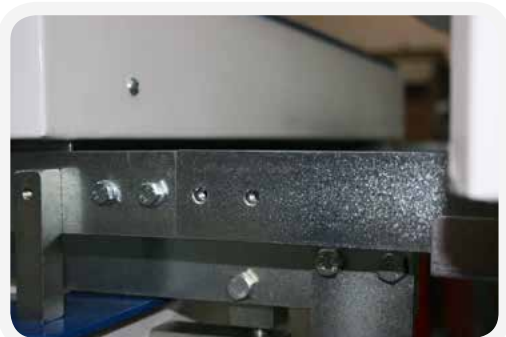
Slide the heater guard onto the links (2 people are required to perform this lift)
