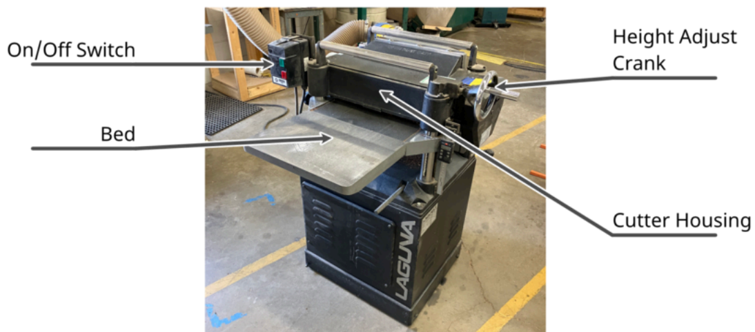
Figure 8: An annotated front quarter view of the planer.
