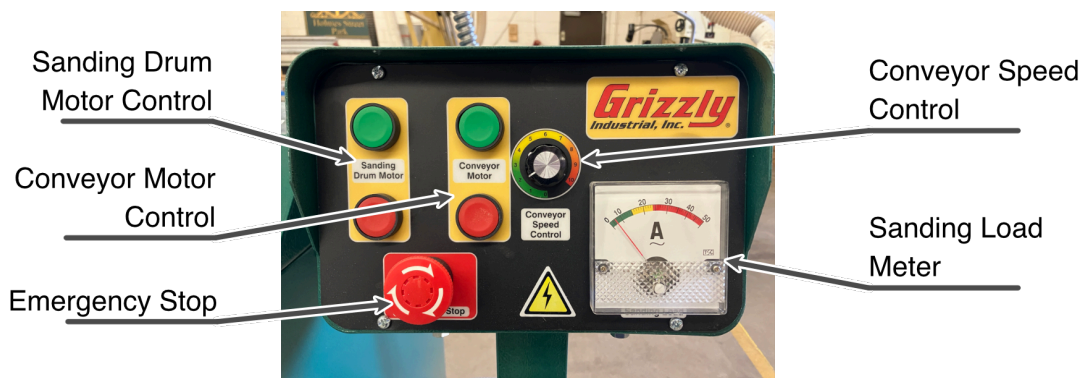
Figure 10: An annotated full view of the drum sander.
