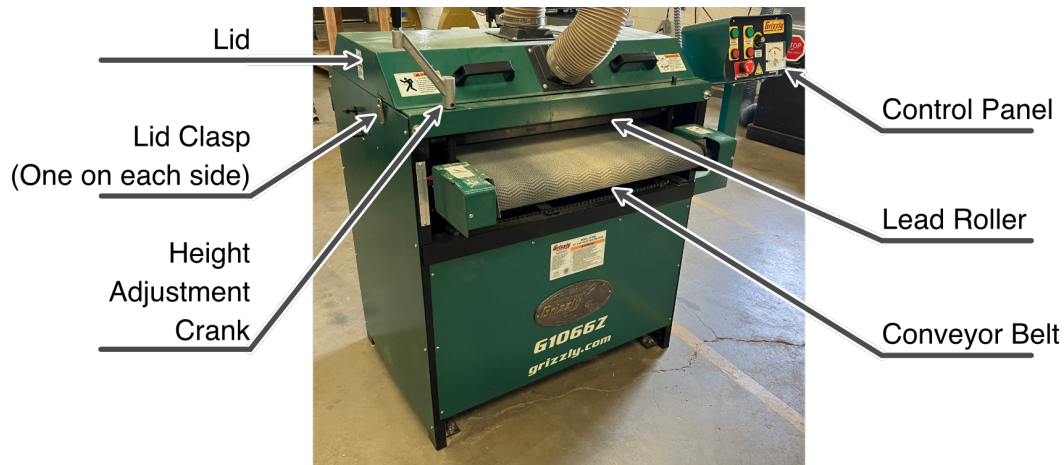
Figure 9: An annotated full view of the drum sander.
