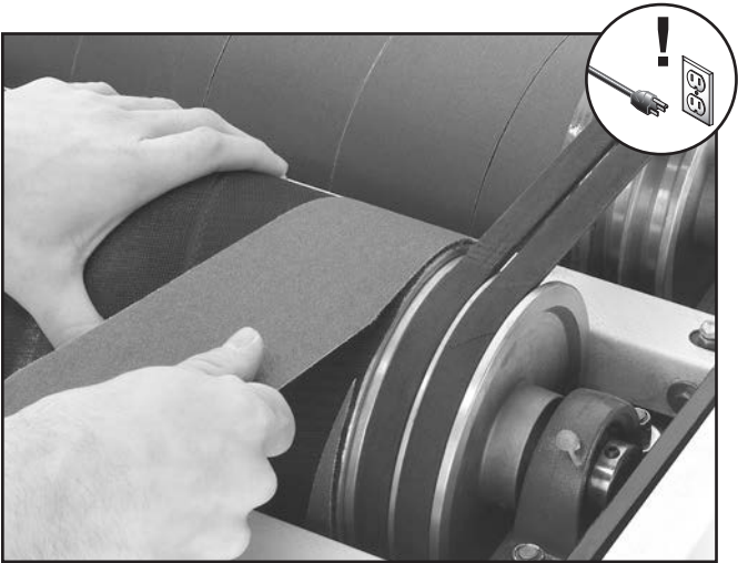
Figure 28. Example of wrapping sandpaper around drum.
