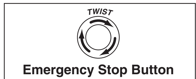
Figure 20. Resetting Emergency Stop button.
