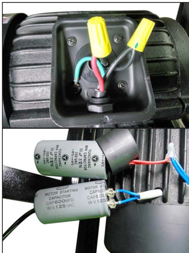
Figure 57. G1066Z drum motor connections and capacitors.
