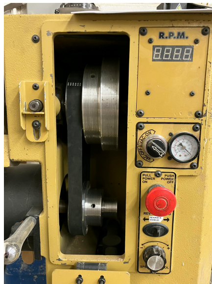
Figure 5: The wood lathe drive belt in the high setting position.
