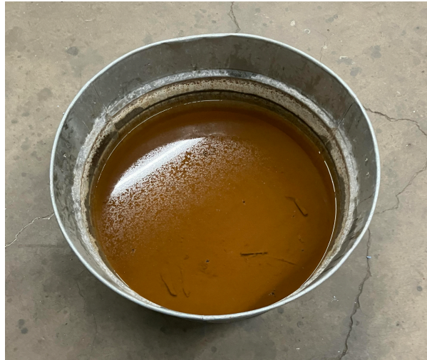
Figure 4: The quench tub on the floor of the blacksmithing area.
