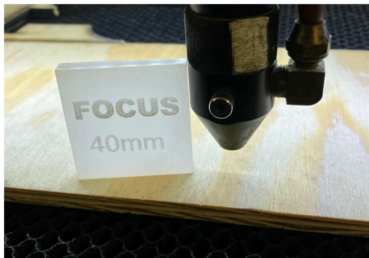
Figure 3: Lens carriage aligned with the focus gauge (40mm).
