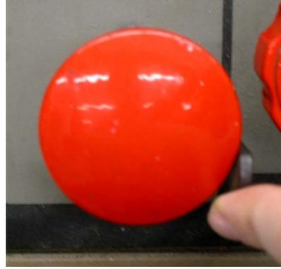
While holding the interlock up, pull the orange knob in until the table plate is lowered to the desired height
