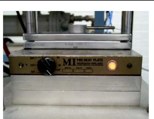
Plug in Hot Plate, and set temperature to desired set point
