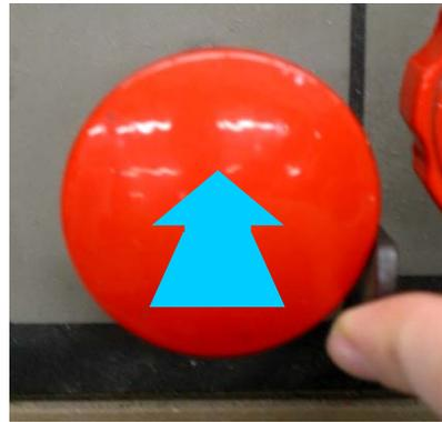
Release the interlock to maintain the table plate at the desired height
