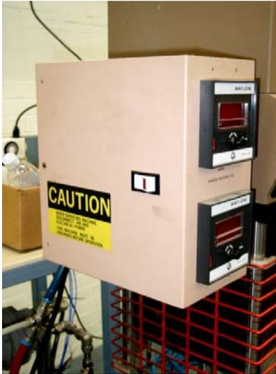
Determine the proper temperatures needed for your material. Use the temperature chart or manufacturer information. Tests may also be performed to determine optimum temperatures to properly melt the material.
