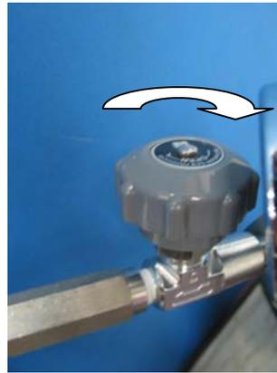
Open the compressed air valve slightly
