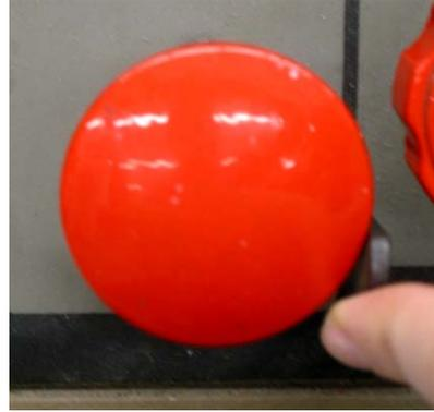
While holding the interlock up, push the orange knob in until the table plate is at the desired height
