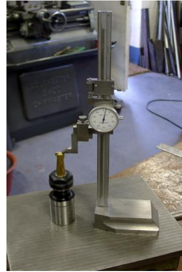
Figure 5.3 – TTS presetting
