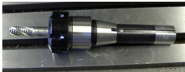
Figure 5.6 – ER32 collet tool holder
