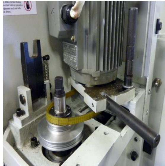
Figure 5.8 – Changing spindle speed range
