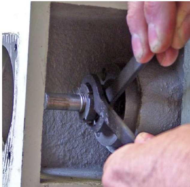
Figure 9.7 – Tightening the lock nut
