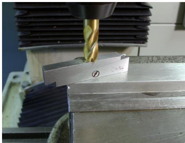
Figure 6.14 – Parallel adjusted to gap
