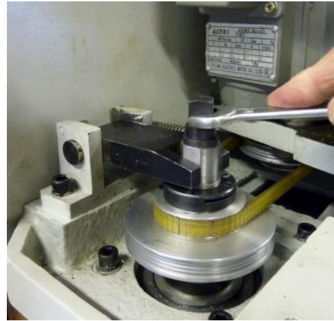
Figure 5.7 – Spindle lock fork engaged
