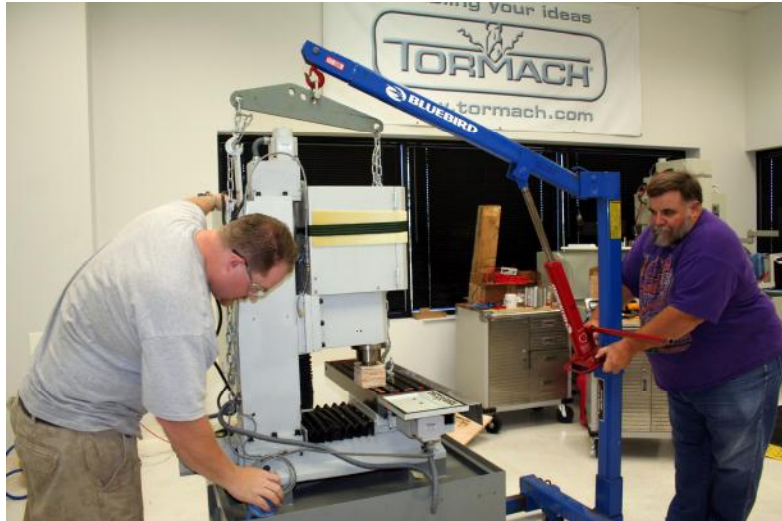
Figure 2.5 – Hoist bar for slinging the mill
