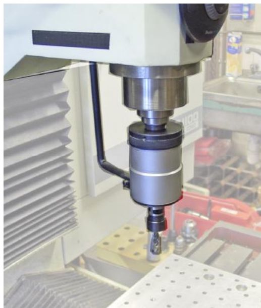
Figure 8.23 – Large tapping head ready for use
