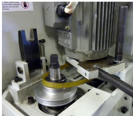
Figure 2.15 – Changing spindle pulley setting
