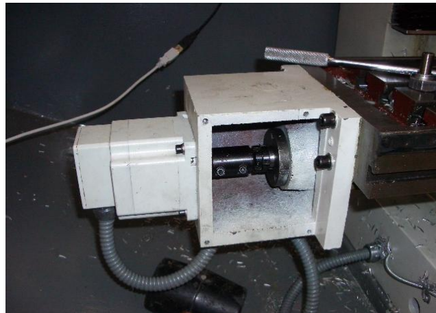
Figure 9.2b – Photograph of X-axis mount
