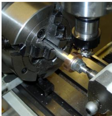
Figure 8.3 – Gear cutting
