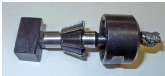
Figure 8.24 – Tap collet and anti-rotation block
