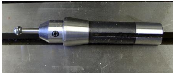
Figure 5.4 – R8 tool-holder
