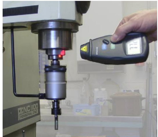
Figure 8.27 – Measuring spindle speed
