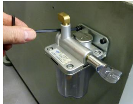
Figure 2.8 – Fitting manual oiler
