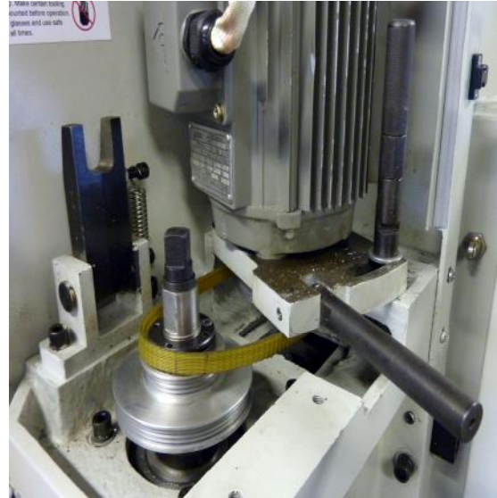
Figure 5.8 – Changing spindle speed range
