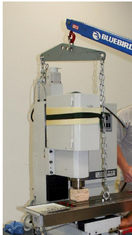
Figure 2.6 – Slinging geometry
