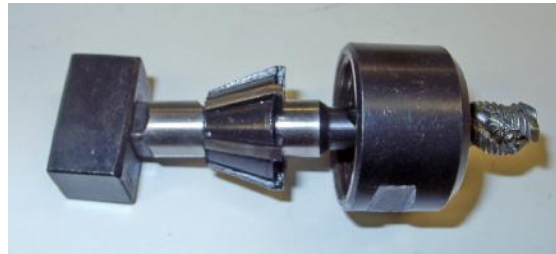
Figure 8.24 – Tap collet and anti-rotation block
