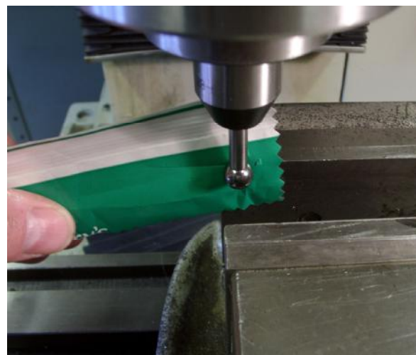
Figure 6.22 – Measuring vise jaw Y position
