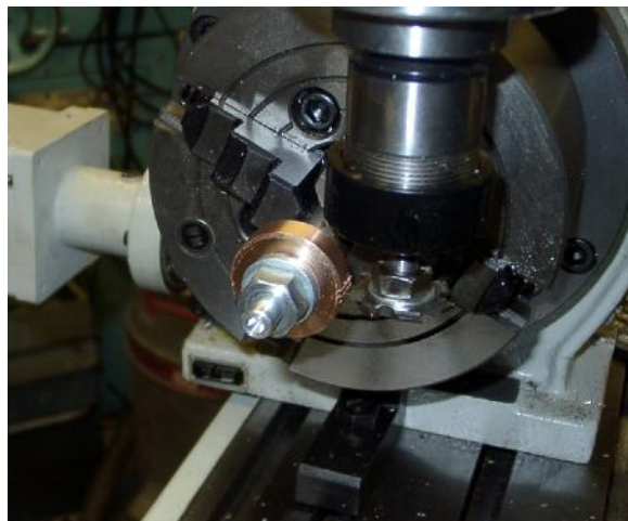
Figure 8.4 – Gear cutting (tailstock removed for clarity)
