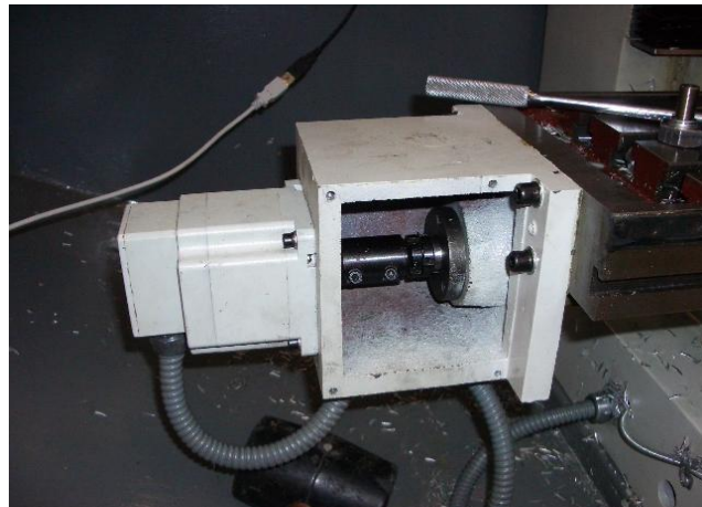
Figure 9.2b – Photograph of X-axis mount
