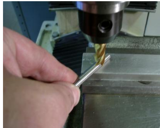
Figure 6.13 – Gauge just rolls under tool
