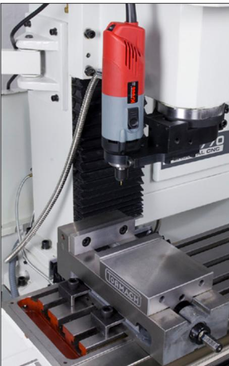
KRESS 800 WATT HIGH SPEED SPINDLE KIT
