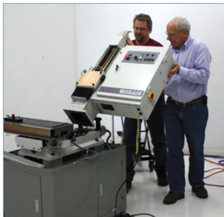
A PATENT-PENDING MOVING KIT MAKES DISASSEMBLY OF THE PCNC 770 SAFER AND EASIER.
